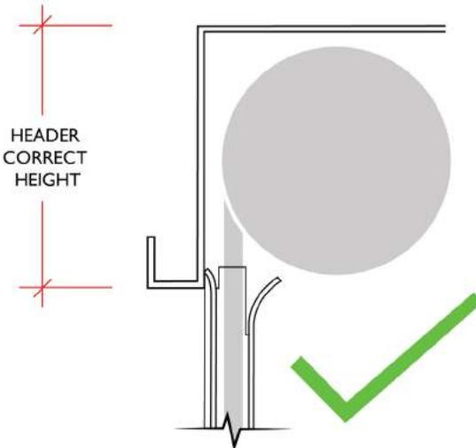
If a shutter is installed incorrectly, it will suffer wear and tear quicker than a well installed shutter.
