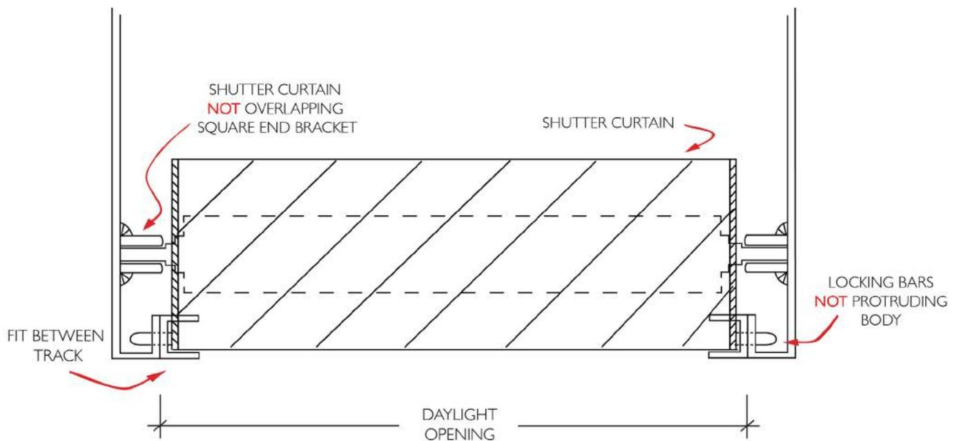
TOP VIEW - **FIT BETWEEN** TRACKS WITH 25mm SIDE ROOM
